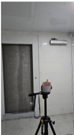
ACOUSTICAL TESTING > 33 R'W
