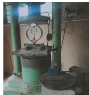
3-POINT BENDING TEST SETUP
