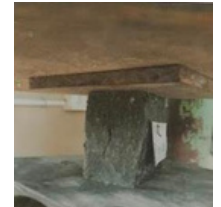
BULGING AT MAXIMUM LOAD
