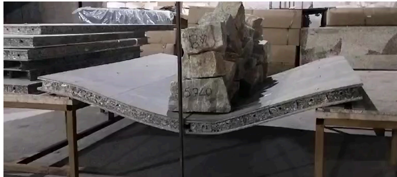
EXTERME WIND LOAD SIMULATION 1000kgs/m 2
