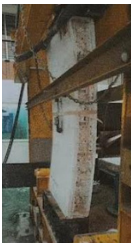
TEST SETUP OF WALL PANELS WITH TRIPLE CEMENT BOARD
