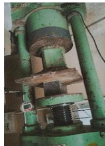
TEST SETUP FOR COMPRESSIVE FORCE PERPENDICULAR TO CEMENT BOARD
