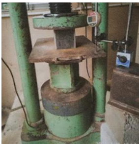
TEST SETUP OF COMPRESSIVE FORCE PARALLEL TO CEMENT BOARD
