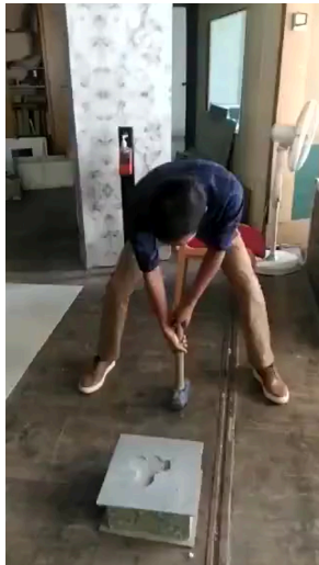
DESTRUCTIVE TESTING Sledge Hammer test
