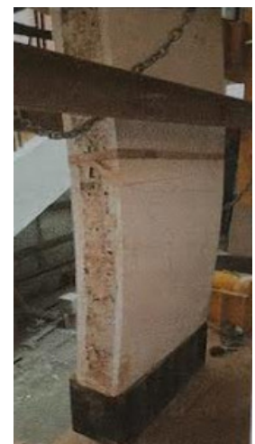
TEST SETUP OF WALL PANELS WITH SINGLE CEMENT BOARD
